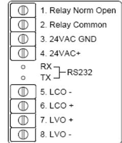
Fig 2: Wiring Connection
